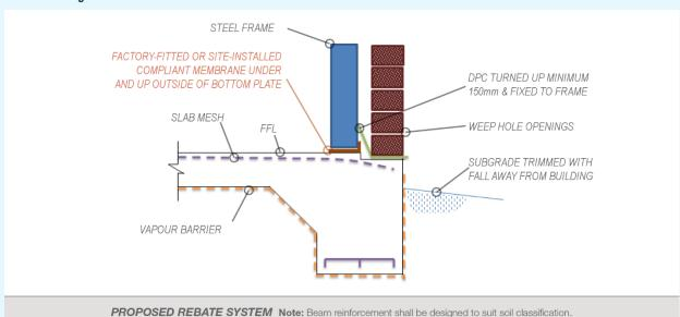
The protection of the weather side flange (see Figures 1 and 2) is necessary because this part of the frame is subject to moist air within the lower parts of the cavity.
